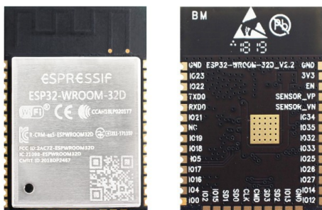
图 2: ESP32-WROOM-32D module (front and back)
