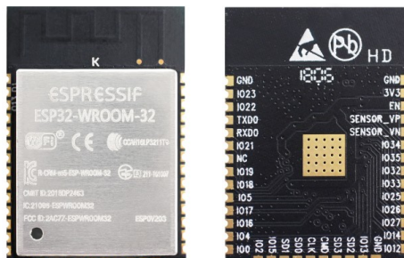
图 1: ESP32-WROOM-32 module (front and back)
